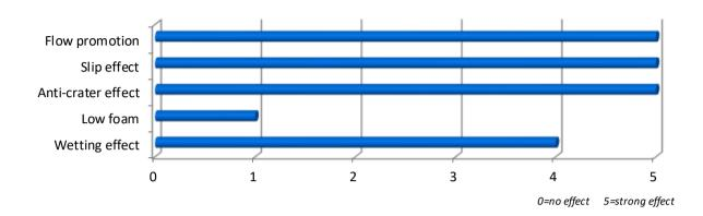
**UNIQ** \*FLOW 493 U is modified polyether polysiloxane leveling agents. The additive gives strong surface tension reduction properties in coatings. The substrate wetting is improved and therefore can also act as an anti-crater agent. **UNIQ** \*FLOW 493 U gives strong surface slip and can help to increase the gloss. In aqueous systems it improves the anti-blocking properties
